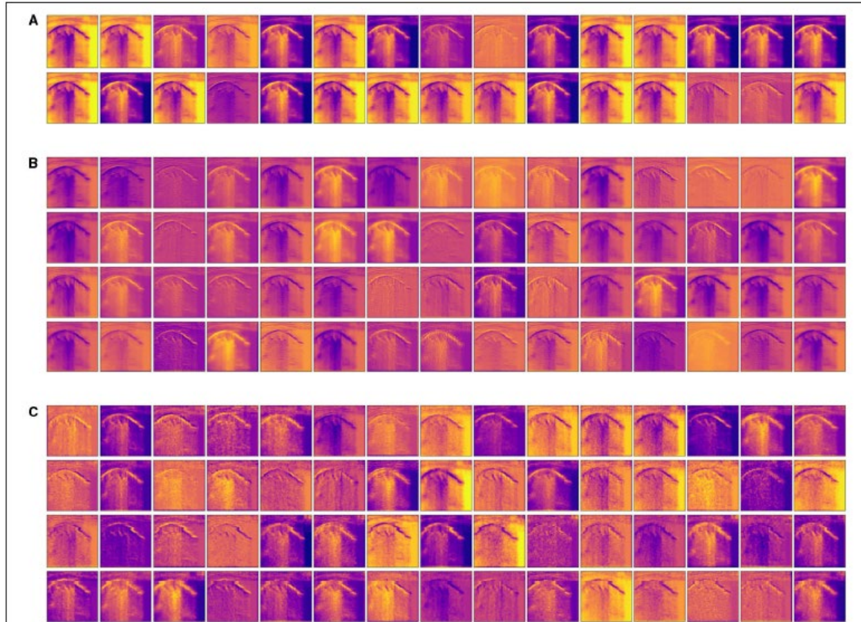
FIGURE 4 | Visualization of the activation maps from (A) the first, (B) the third, and (C) the fourth convolutional layer of the best performance model (Inception-v3) on the three-class classification problem, when fed with an image of a lung with bronchiolitis. Filters act as collections of edge detectors, detect background, contours, and texture-like patterns. When going deeper in the layers, the filters enhance differently vertical artifacts and small consolidation-like patterns that are typical of bronchiolitis.
